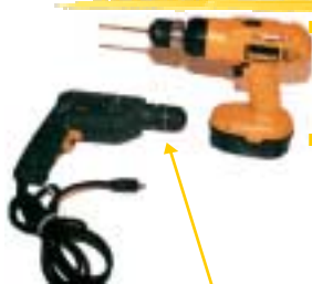
Note: Keyless chuck (next slide shows a keyed chuck)
