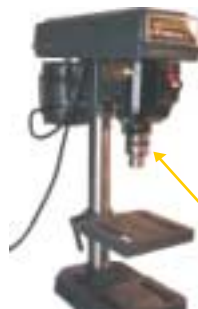
Note: Keyed chuck to grip the bit
